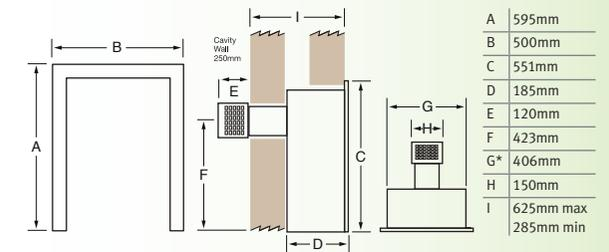
Dimensions A & B refer to Profiled trim only. \*Dimensions differ on Easy Flame control models. Please refer to installation manual. An optional flue extension is available to increase the maximum flue length to 1010mm on manual models and 973mm on Easy Flame models.
