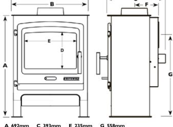
A 692mm C 393mm E 235mm G 558mm B 523mm D 357mm F 160mm
