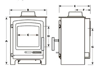
C 260mm E 346mm G 463mm **D 237mm F 163mm** (138mm using optional flue casting collar)
