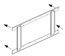
Fix bracket to wall using suitable size screws and wall plugs appropriate for the walls construction. Note heavy duty wall anchors or equivalent should be used when installing onto hollow/studded walls.
