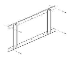
Hang the appliance onto the hooks at the bottom of the bracket and push the top of the appliance into the mounting bracket. Now fix the appliance to the mounting bracket by refitting the two screws which were removed at the beginning.
