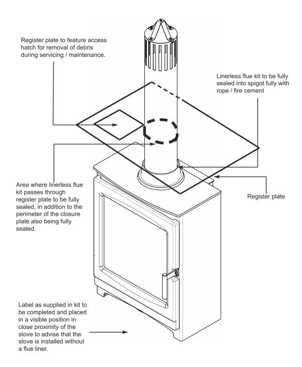
IMPORTANT NOTE: INSTALLATION OF THE LINERLESS FLUE KIT IS SUBJECT TO THESE INSTRUCTIONS BEING STRICTLY ADHERED TO AND TO COMPLETION OF A SATISFACTORY SPILLAGE TEST AS DETAILED IN THE MAIN INSTRUCTION MANUAL.
