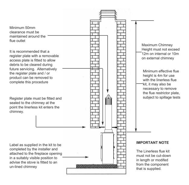
The product should be installed as displayed below in figure 2.
