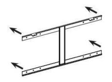
Fix bracket to wall using suitable size screws and wall plugs appropriate for the walls construction. Note heavy duty wall anchors or equivalent should be used when installing onto hollow/studded walls.
