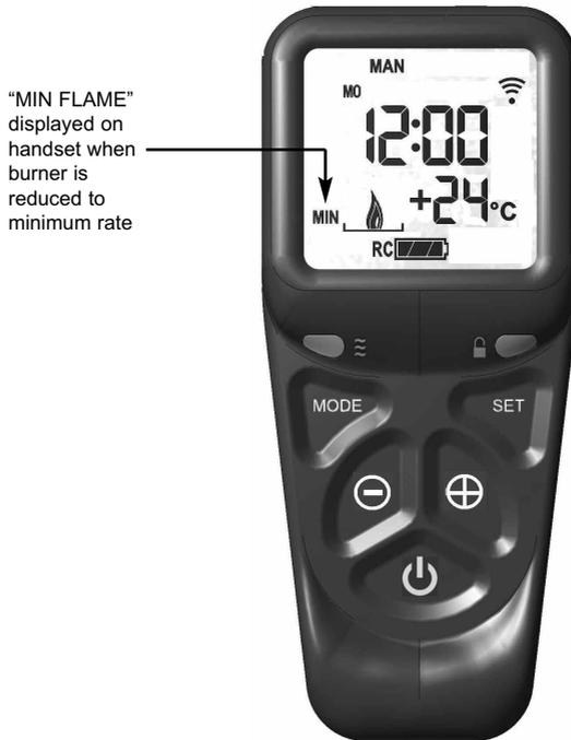
5.3.4 To increase the heat input level of the fire's burner hold the handset as described in section 5.3.1 to unlock the keypad then press and release the + button. Pressing and releasing the + button will increase the heat input level one step at a time. Pressing the + button continuously will move the heat input level to the maximum.
