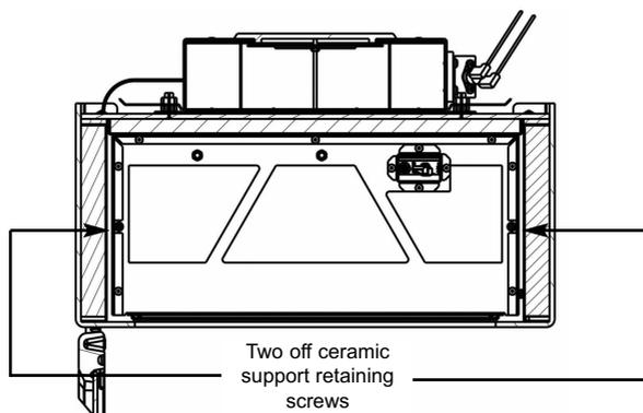
4.1.3 Remove the 4 off screws that hold the burner in position, see figure 30 below.
