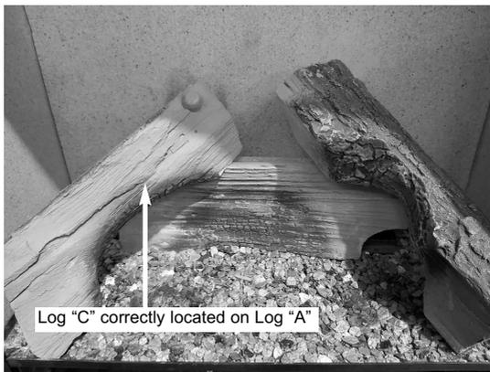
3.1.5 Place log "C" onto the groove in the centre of the base ceramic log as shown below in figure 16.
