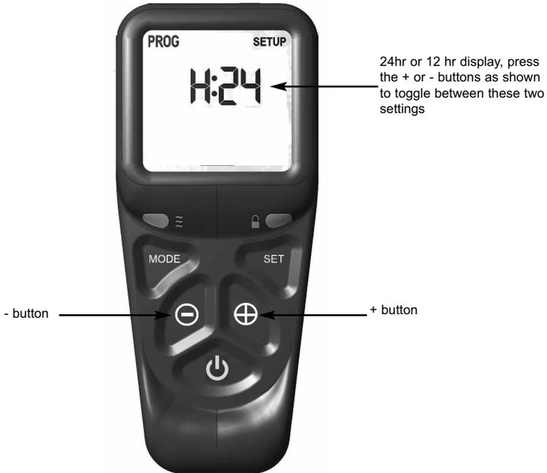
3.3.4 When the 24hr or 12hr time display option has been chosen and you are ready to confirm the setting you want press the SET button on the handset to progress to setting the day of the week as shown overpage in figure 17.
