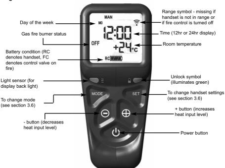
3.4.2 Press and hold the power button continuously until the word "PILOT" appears at the bottom left of the display as shown overpage in figure 22, (this typically takes two seconds). The burner will now light at maximum heat input level and will display "MAX" in the bottom left hand side of the display as shown in figure 23 overpage.
