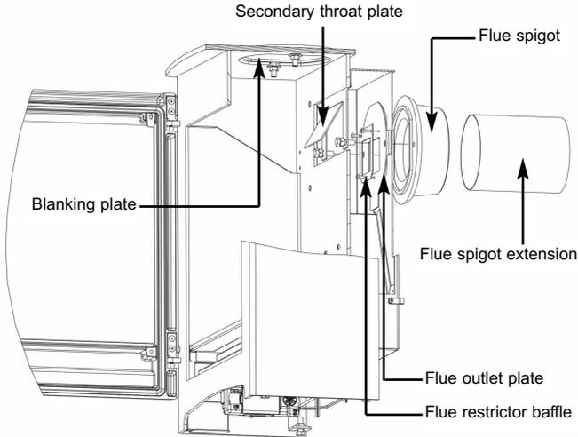
**IMPORTANT NOTE : WHEN SETTING UP THE STOVE TO USE A REAR FLUE CONFIGURATION THE SECONDARY THROAT PLATE WHICH IS IDENTIFIED ABOVE IN FIGURE 6 AND SUPPLIED IN THE LOOSE ITEMS PACK MUST BE FITTED. THE STOVE MUST NOT BE INSTALLED ON A REAR FLUE CONFIGURATION WITHOUT THIS COMPONENT FITTED. A SPILLAGE TEST MUST BE PERFORMED ON REAR FLUE CONFIGURATIONS.**
