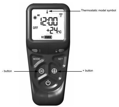
5.7.2.3 Press the set button again to see the temperature setting that is set (the default is 24 degrees celsius). If a different set temperature is required, whilst the display is showing this set temperature, press the + and - buttons to alter this setting, press the set button to store the required temperature, or alternatively the handset can be left for a few seconds and the temperature will be stored automatically.
