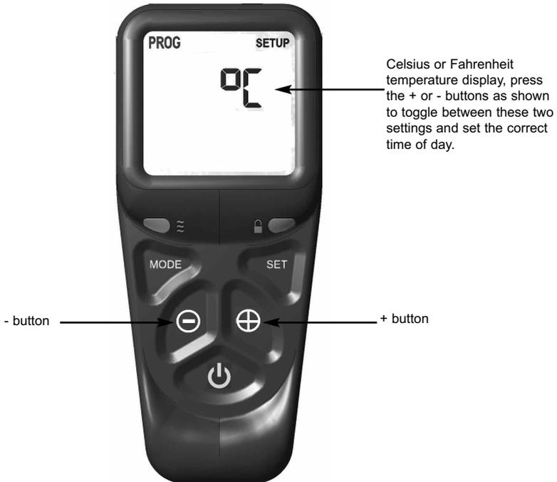
3.3.7 As shown above in figure 20 the time on the handset can now be set by using the + and - buttons to change the hour to the correct hour then press SET to store and to move to setting the minute. Repeat this process for setting the minute to the correct minute then press SET to store.
