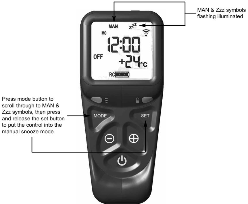
3.5.1.6 Pressing the set button again will now show you the snooze time period remaining. The snooze time period can be adjusted by pressing the + or - buttons on the handset. This time period can be set ranging from 1 minute to 4:00 hours.
