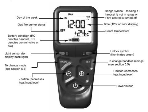
5.3.2 Press and hold the power button continuously until the word "PILOT" appears at the bottom left of the display as shown overpage in figure 2, (this typically takes two seconds). The burner will now light at maximum heat input level and will display "MAX" in the bottom left hand side of the display as shown in figure 3 overpage. For most efficient performance leave the fire on high when lighting from cold for ten minutes.
