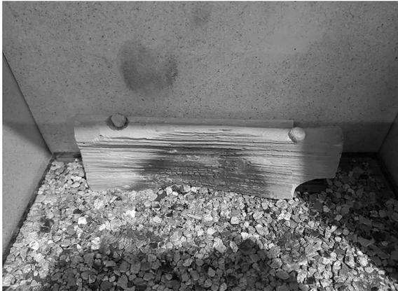
5.9.3 Position Log "B" onto Log "A" as shown below in figure 18, using the locating lug on Log "A" and the locating point on Log "B" as a guide for placement as shown below in figure 18.
