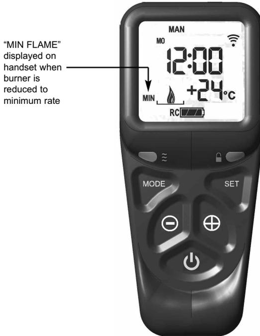
3.4.4 To increase the heat input level of the fire's burner hold the handset as described in section 3.4.1 to unlock the keypad then press and release the + button. Pressing and releasing the + button will increase the heat input level one step at a time. Pressing the + button continuously will move the heat input level to the maximum.
