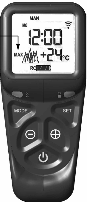
Fig. 45 - “MAX” & large flame symbol displayed
