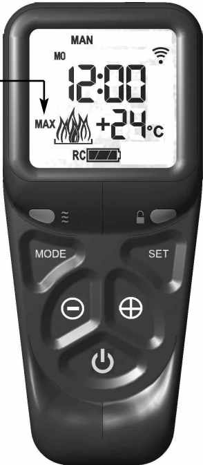
Fig. 3 - “MAX” & large flame symbol displayed
