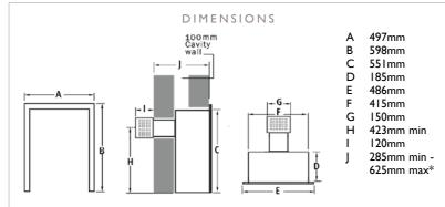
\*Dimensions differ on EFC models. An optional flue duct extension is available to increase maximum length to 1015mm on manual models and 973mm on EFC models.
