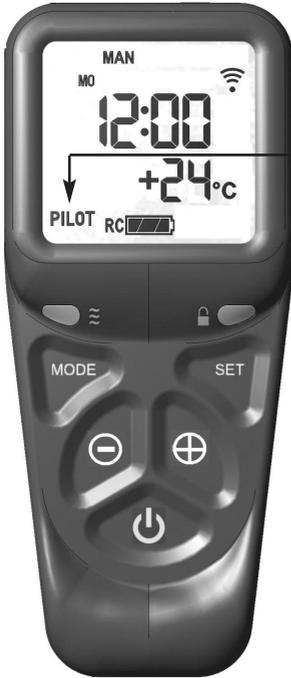
"PILOT" displayed on handset during ignition sequence (typically takes two seconds)
