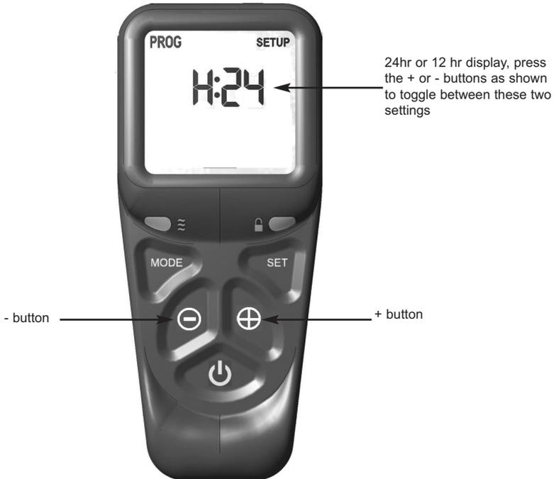
3.3.4 When the 24hr or 12hr time display option has been chosen and you are ready to confirm the setting you want press the SET button on the handset to progress to setting the day of the week as shown overpage in figure 21.
