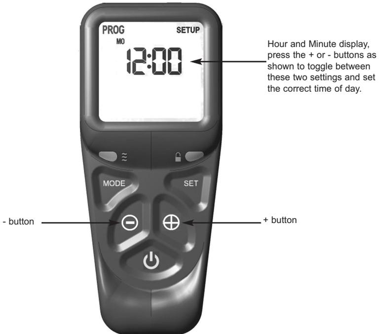
5.6.7 As shown above in figure 10 the time on the handset can now be set by using the + and - buttons to change the hour to the correct hour then press SET to store and to move to setting the minute. Repeat this process for setting the minute to the correct minute then press SET to store.
