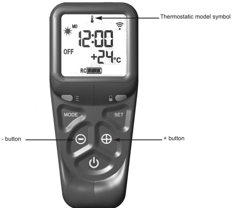
3.5.2.3 Press the set button again to see the temperature setting that is set (the default is 24 degrees celsius). If a different set temperature is required, whilst the display is showing this set temperature, press the + and - buttons to alter this setting, press the set button to store the required temperature, or alternatively the handset can be left for a few seconds and the temperature will be stored automatically.
