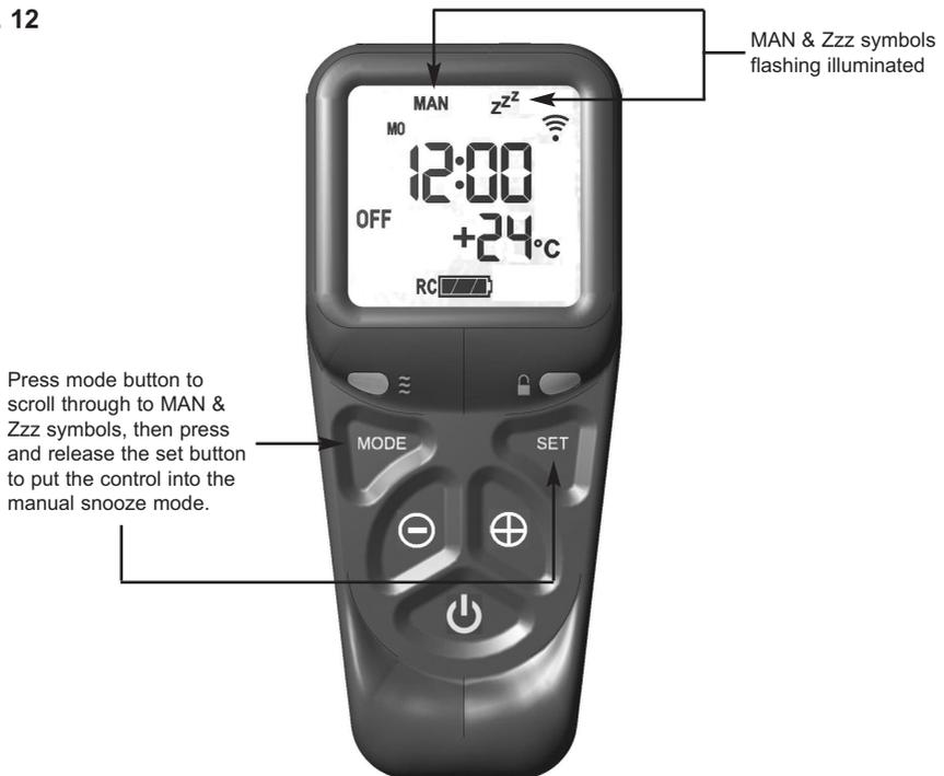
5.7.1.6 Pressing the set button again will now show you the snooze time period remaining. The snooze time period can be adjusted by pressing the + or - buttons on the handset. This time period can be set ranging from 1 minute to 4:00 hours.
