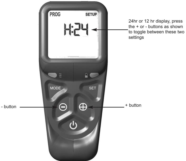
5.6.4 When the 24hr or 12hr time display option has been chosen and you are ready to confirm the setting you want press the SET button on the handset to progress to setting the day of the week as shown overpage in figure 10.
