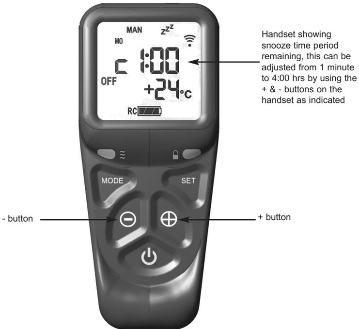
5.7.1.8 To adjust the snooze period use the + and - buttons to increase or decrease the snooze period for any period between 1 minute and 4:00 hours.
