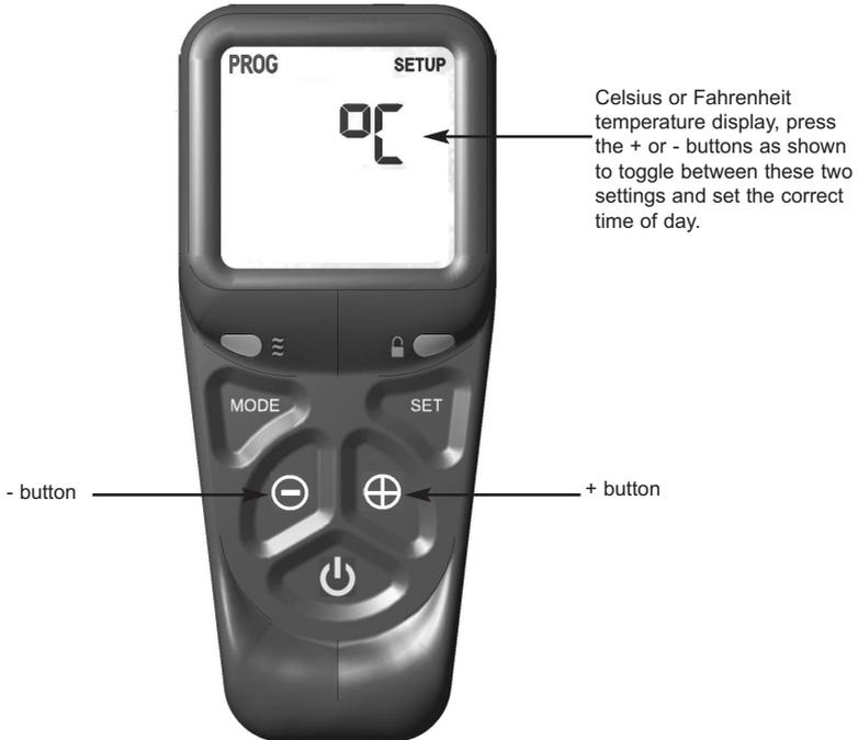
3.3.7 As shown above in figure 21 the time on the handset can now be set by using the + and - buttons to change the hour to the correct hour then press SET to store and to move to setting the minute. Repeat this process for setting the minute to the correct minute then press SET to store.
