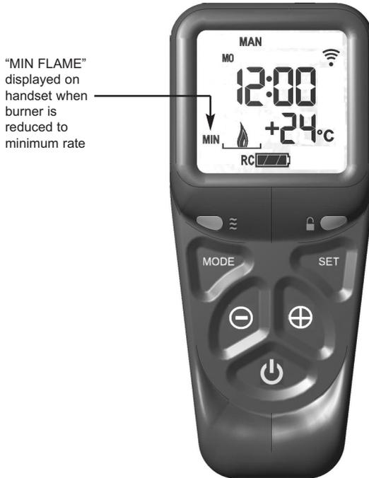
3.4.4 To increase the heat input level of the stove's burner hold the handset as described in section 3.3.2 to unlock the keypad then press and release the + button. Pressing and releasing the + button will increase the heat input level one step at a time. Pressing the + button continuously will move the heat input level to the maximum.
