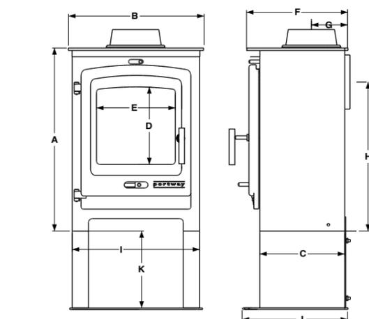
A 588mm C 260mm E 247mm G 112mm I 390mm K 250mm
