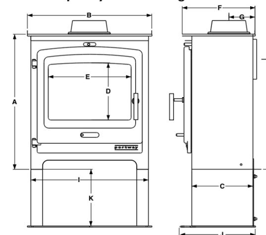
A 588mm C 260mm E 350mm G 112mm I 500mm K 250mm
