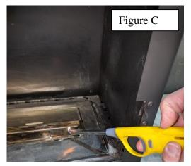
residual heat. **Caution is advised**, as the ignition will likely be more 'instant' with a larger flame, once lit, adjust the slider if desired, then immediately close the door. If the burner does not relight, it is either empty or does not have enough residual heat to reignite, in this case, you must allow the burner to cool before attempting to refill.
