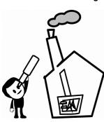
CHECK FOR SMOKE: Apart from a little, mostly harmless steam, when cold and first lit, there should barely be any visible smoke from the chimney. How to achieve this will depend on the fuel, air control and the way you use the stove. Check the enclosed Smoke Leaflet, or download an extra copy from www.soliftec.com
