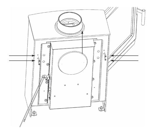
5.) Remove the ceramic fuel tray support brackets (L/H & R/H) from the stove, secured with 2 off screws per side as shown below in figure 5
