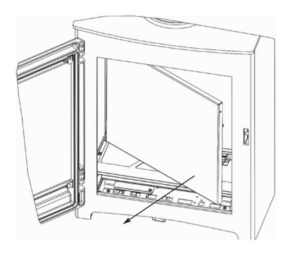
3.) Remove the ceramic fuel tray from the stove as shown below in figure 3.
