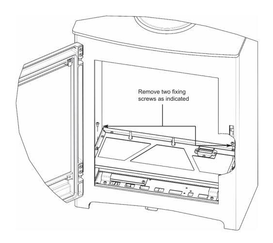
2.) Remove the rear liner from the stove as shown below in figure 2.
