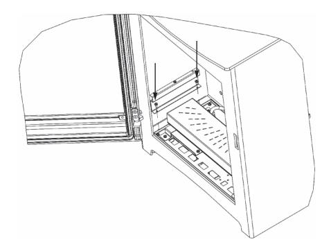
6.) The side liners (L/H & R/H) can now be removed as displayed below in figure 6.
