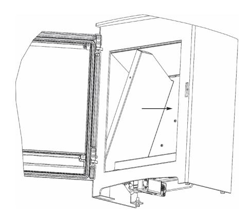
7.) Replace the new liners in reverse order and ensure that the throat plate fixing screws are re-fitted as shown below in figure 7. Ensure also that the rear liner is flush to the rear of the stove.
