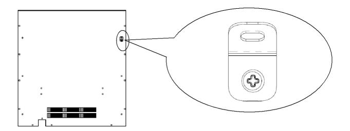
Step 4Drill a hole into the wall and insert the wall plug, fix the other metalbracket to the wall using the screw provided.
