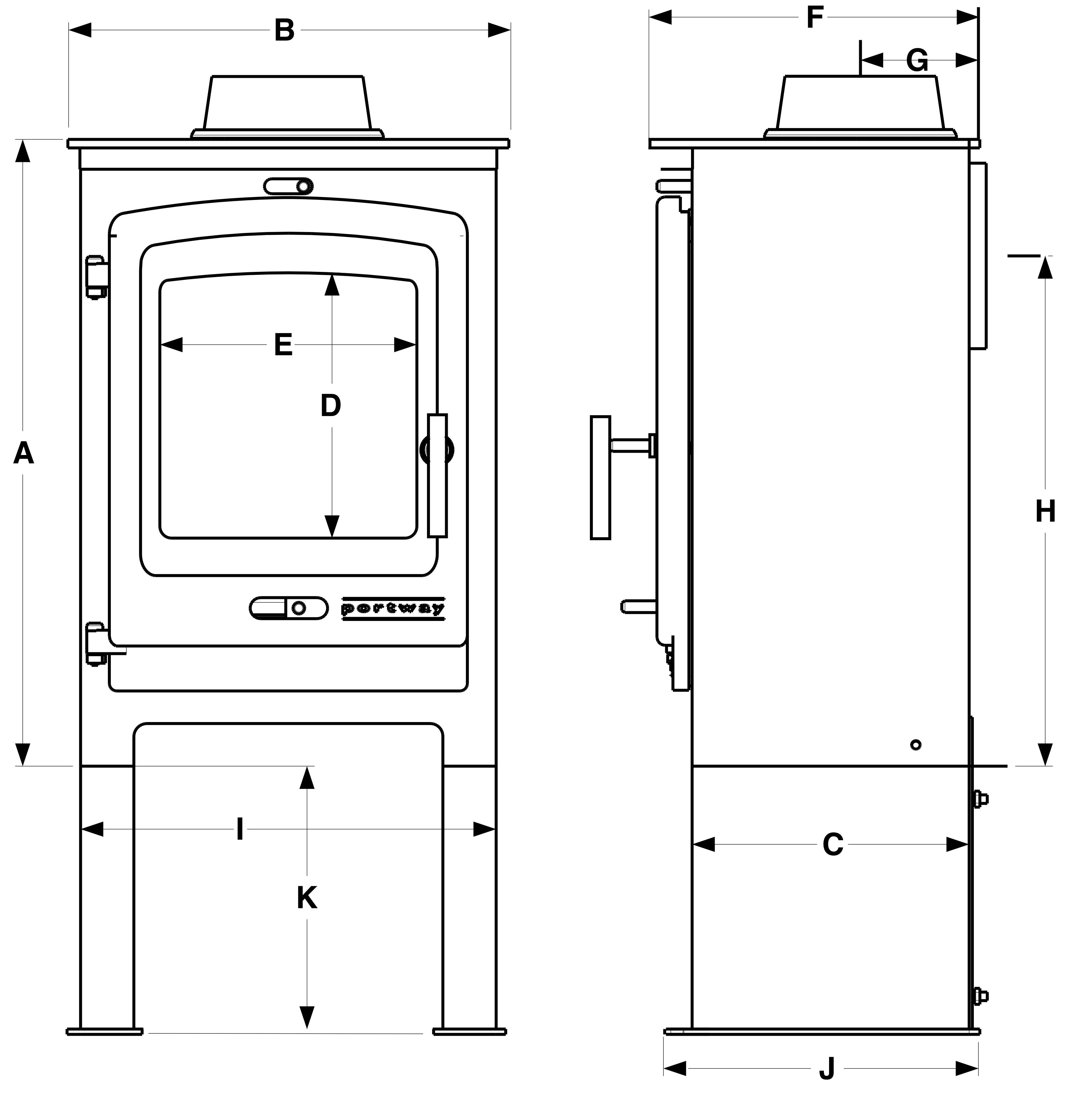
A 588mm C 260mm E 247mm G I 12mm I 390mm K I 50mm Low Legs B 415mm D 254mm F 310mm H 451mm J 310mm 300mm High Legs
