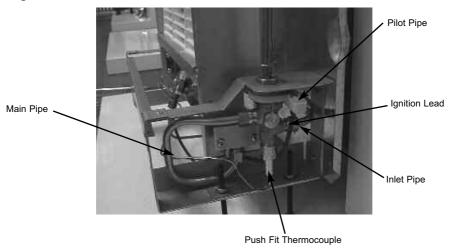
d) Remove the control valve locknut and lift clear.
