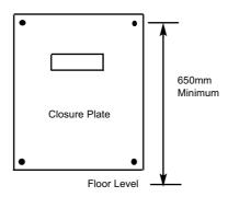
Drill and plug all four holes to take 2 inch No. 10 woodscrews, loosely insert the screws, and place the closure plate in position, sealing it to the wall with 50mm high temperature adhesive on all four sides. Remove the lower screws and screw in the upper ones to leave a 7 to 8mm gap under the heads. Remove the fire feet. Hang the fire on the upper screws, remove the lower screws and tighten all four screws.
