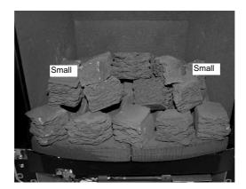
g) Select the remaining two oblong coals, one random coal and one square coal and position along the rear edge of the fuelbed.
