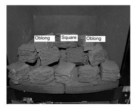
f) Select the two small coals and position to fill the gaps at each end of the third row of coals, (See figure 6 below).
