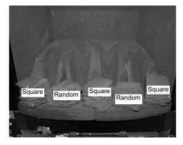
d) Select two of the large square coals two of the large random coals and arrange behind the front row of coals, ensuring that flame paths as indicated below are not interupted, place one of the small coals at each end of the second row. (See figure 4 below).
