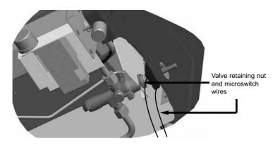
4.4.5 Remove the thermocouple, which is a push fit into the rear of the control valve.
