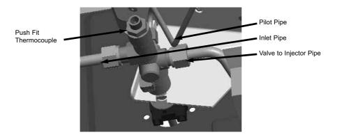
4.4.4 Remove the valve retaining nut as shown below and disconnect the wires to the microswitch as shown below in figure 31
