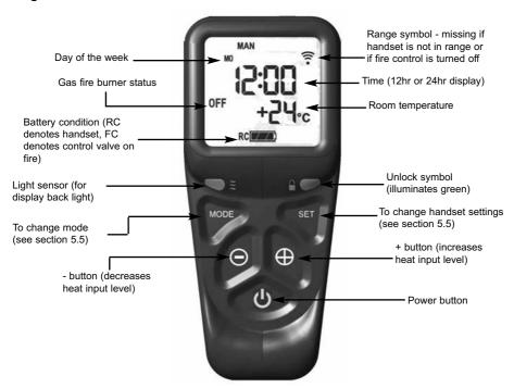
5.2.2 Press and hold the power button continuously until the word "PILOT" appears at the bottom left of the display as shown overpage in figure 2, (this typically takes two seconds). The burner will now light at maximum heat input level and will display "MAX" in the bottom left hand side of the display as shown in figure 3 overpage. For most efficient performance leave the fire on high when lighting from cold for ten minutes.
